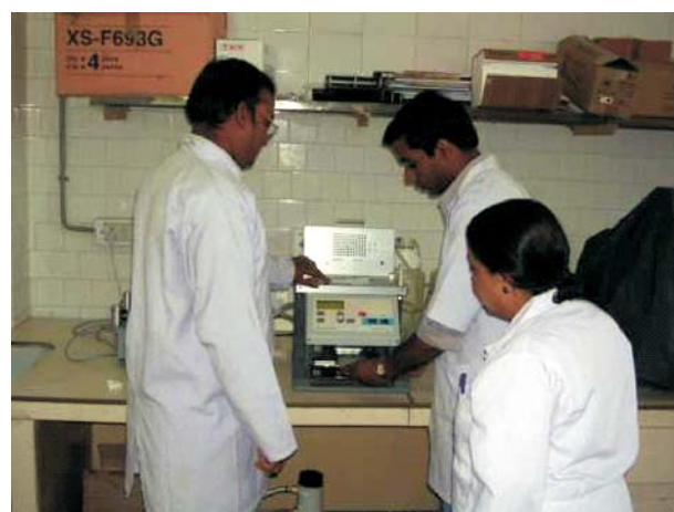
Harvesting of labelled lymphocytes onto glass-fibre filters in Cell Harvester
