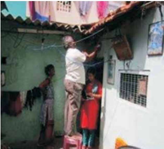
Fig. 4: Placement of 'Hobo' for recording temperature and humidity.
